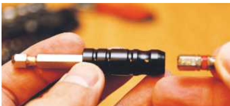
▲ With the black sleeve forwards the standard 6.3mm hex bits are held
